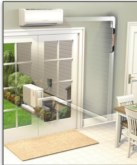
An illustration of a ductless mini-split system.
