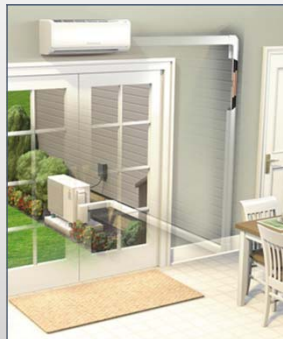
An illustration of a ductless mini-split system.
