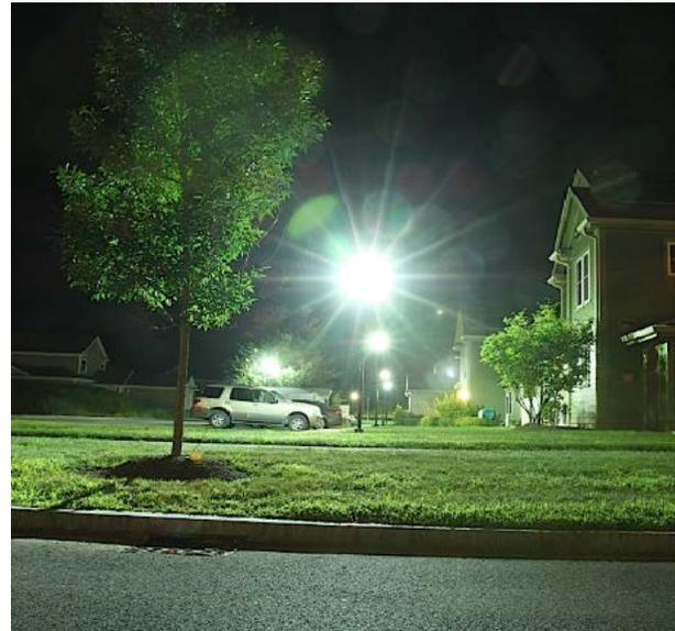
Light pollution and light trespass are both present here in the glare, lack of shielding, stark white color, and spillover of light in all directions and past the property line.
