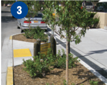
Curb extensions visually and physically narrow the roadway
