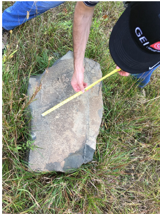
Photo 12 – Rock Slope No. 4: Rockfall from wedge failure, ~STA 16+50, 17 ft from base
