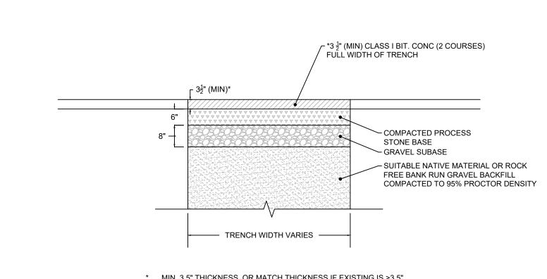
MIN. 3.5" THICKNESS, OR MATCH THICKNESS IF EXISTING IS >3.5"
