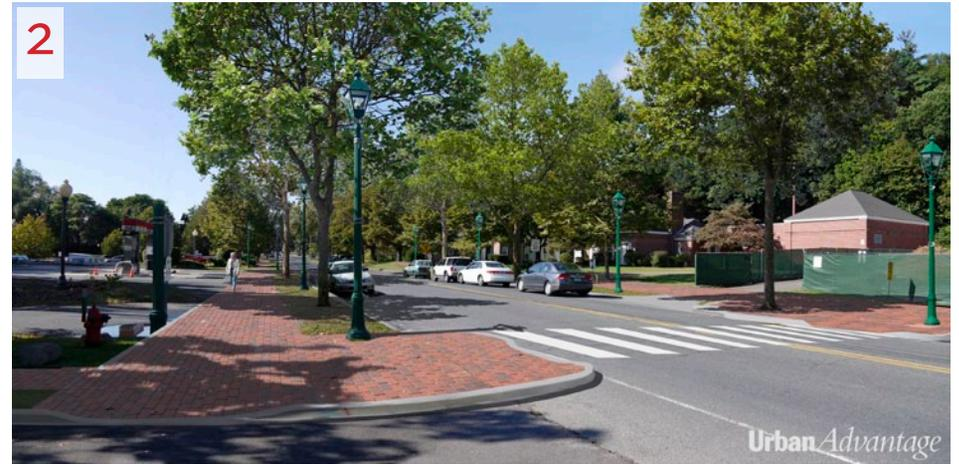
WALKABILITY. Electric lines buried and poles removed, driveway closed, bump outs added, street trees planted and pedestrian-scaled street lighting installed. On-street parking formalized.
