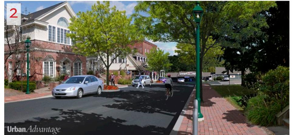
WALKABILITY. Electric lines buried and poles removed, sidewalk widened on south side of street, bump outs added, street trees planted and pedestrian-scale street lighting installed. On-street parking formalized (one side of the street only).
