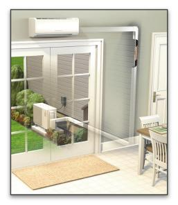
An illustration of a ductless mini-split system.
