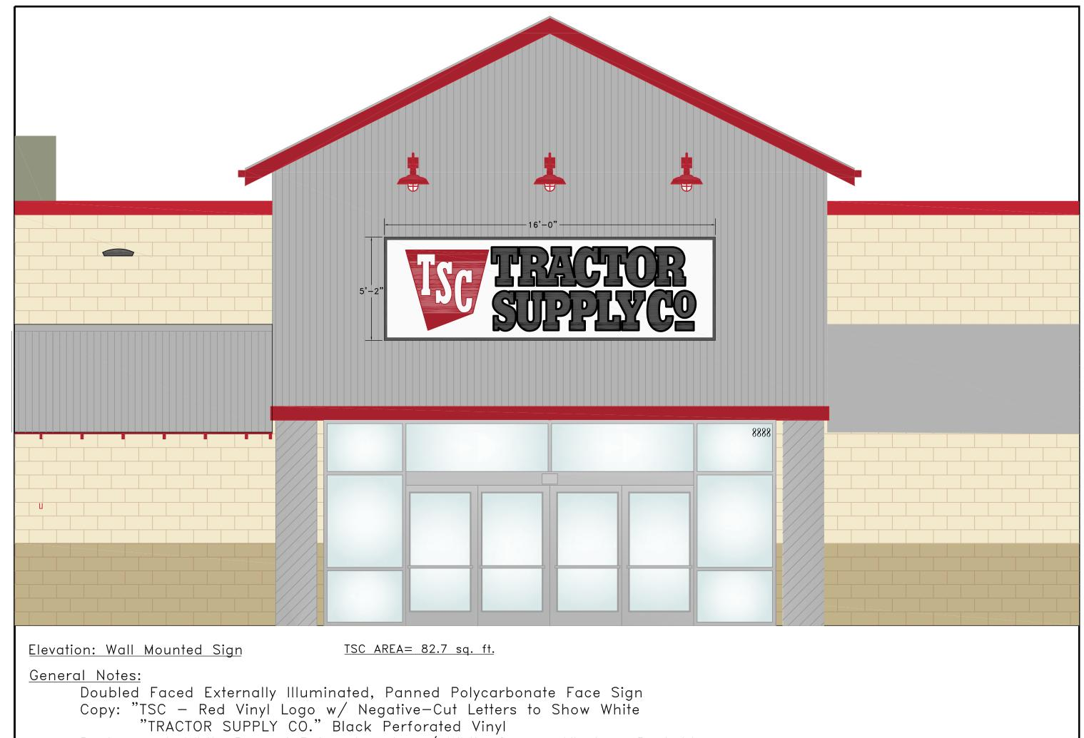
Doubled Faced Externally Illuminated, Panned Polycarbonate Face Sign
