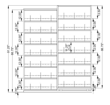
Aurora Side-To-Side -Starter Base includes Deck & Overhead Anti-tip -Adder Base includes Deck, Overhead Anti-tip & Carriage
