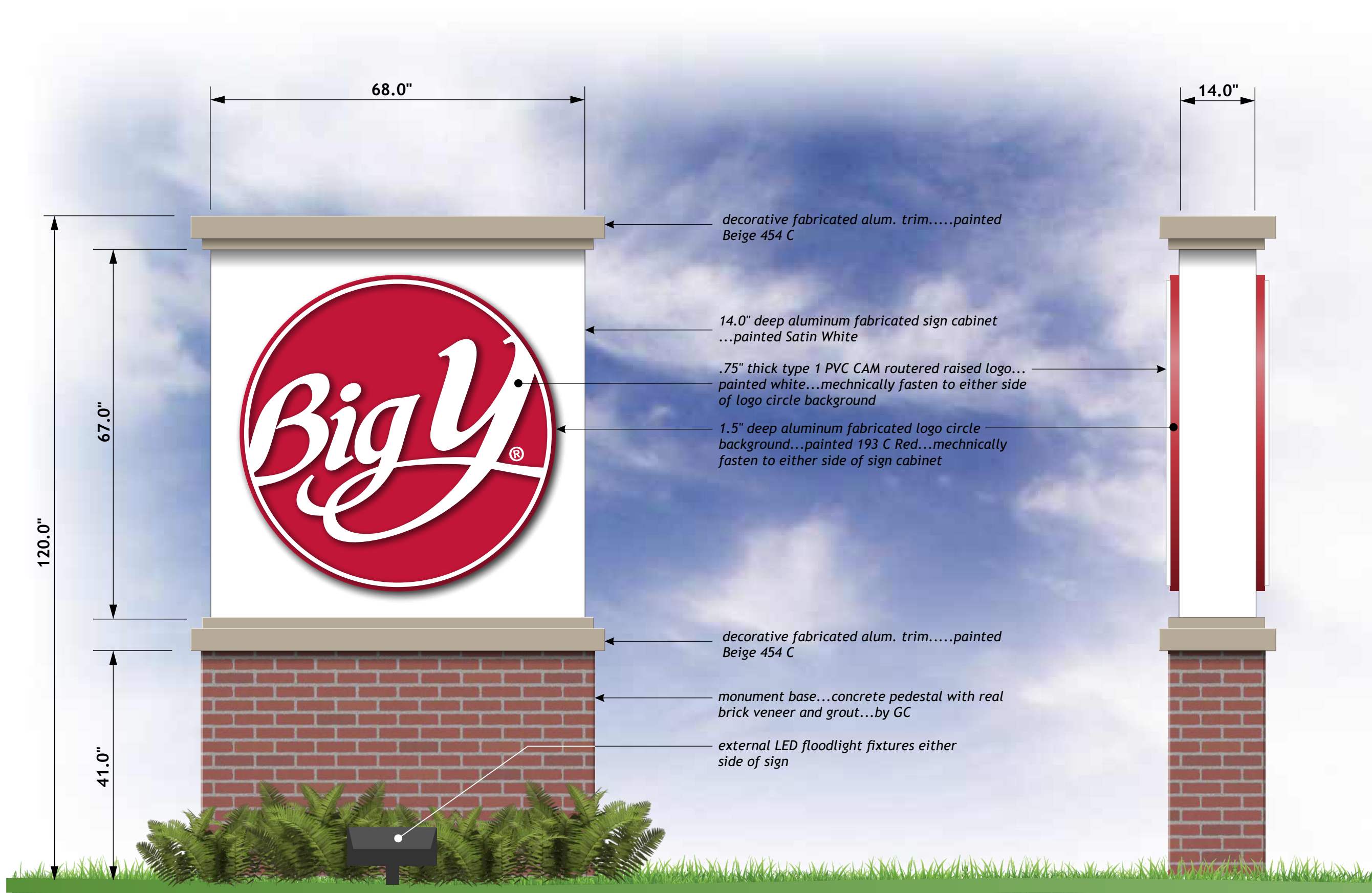
A...(1)...Double Sided Externally Illuminated Monument Sign...NTS...32 sq. ft. area
