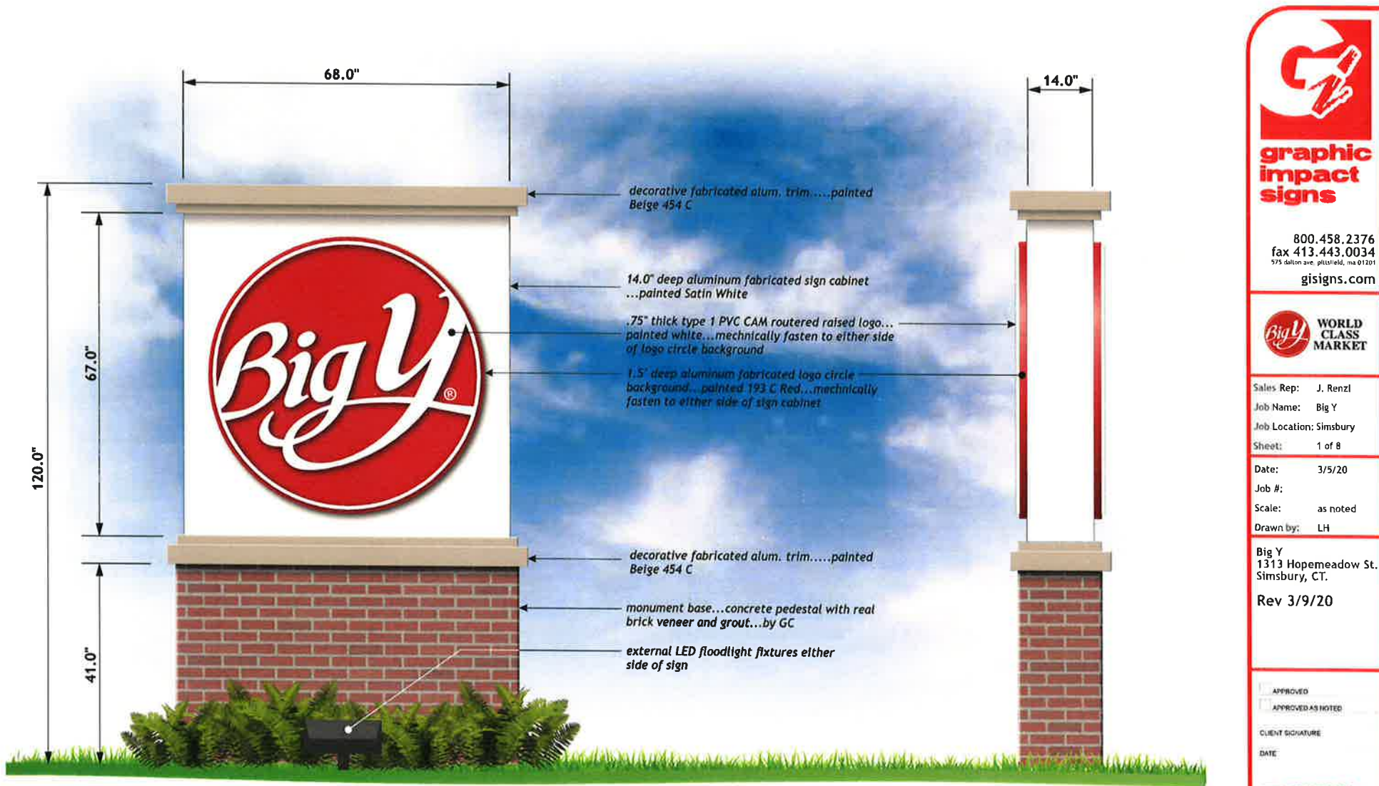
A...(1)...Double Sided Externally Illuminated Monument Sign...NTS...32 sq. ft. area
