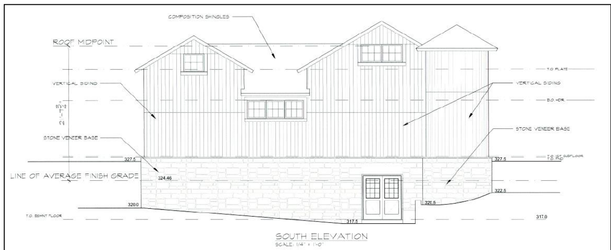
Graphic 3 (Below): South elevation of the proposed barn showing grade.
