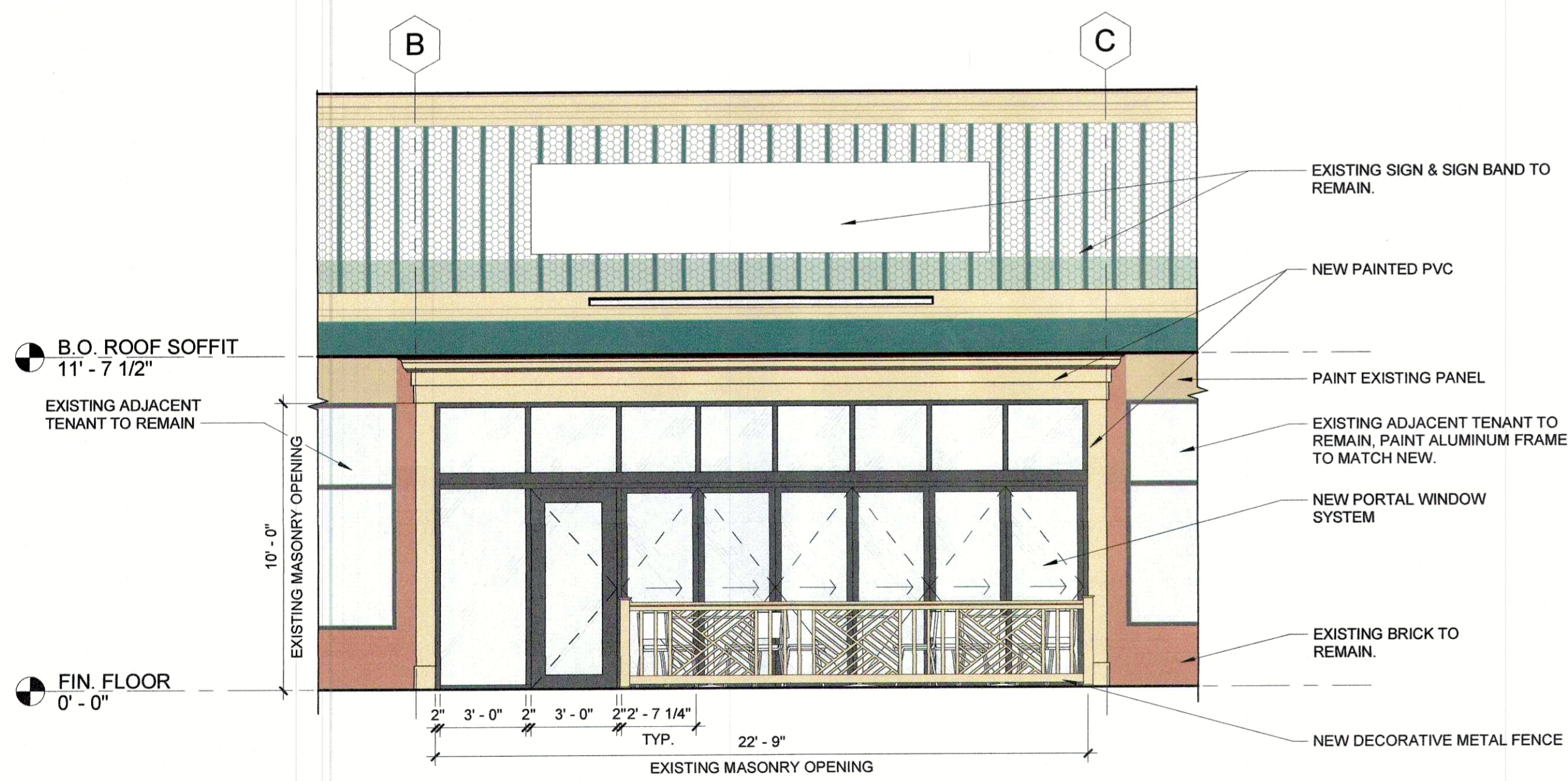
2 PROPOSED ELEVATION SCALE: 1/4" = 1'-0"
