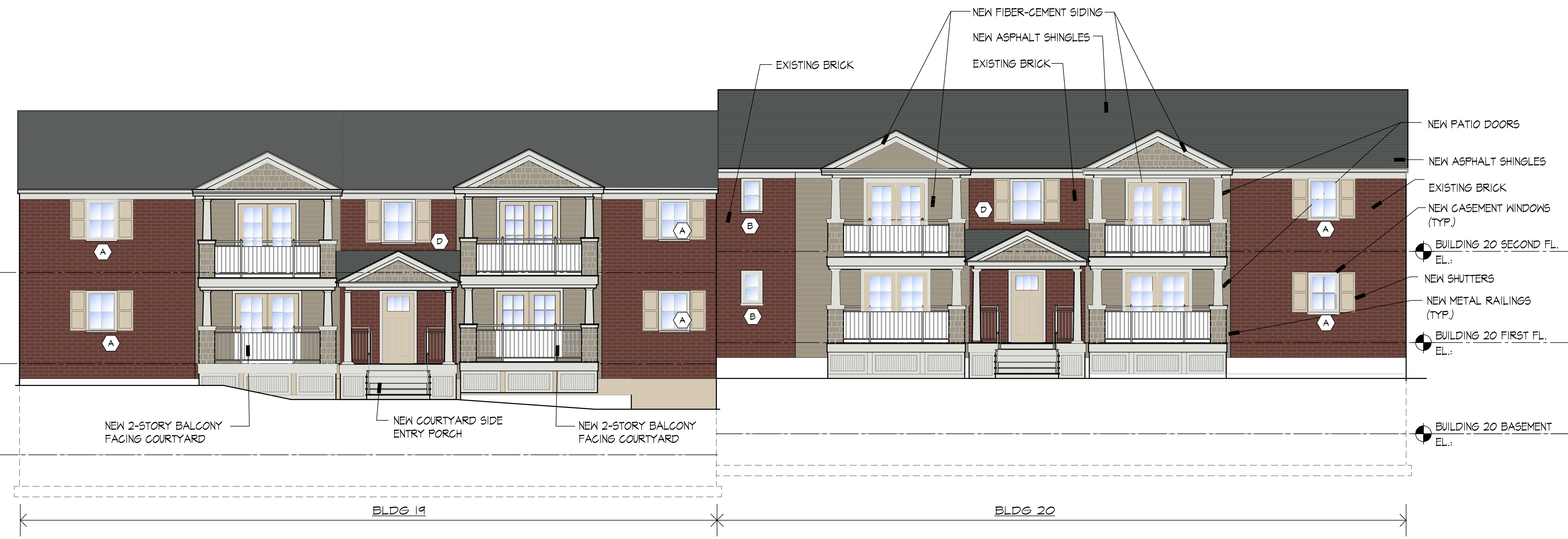
1 EAST ELEVATION BUILDING # 2 A2.2B2 1/8"=1'-0"
