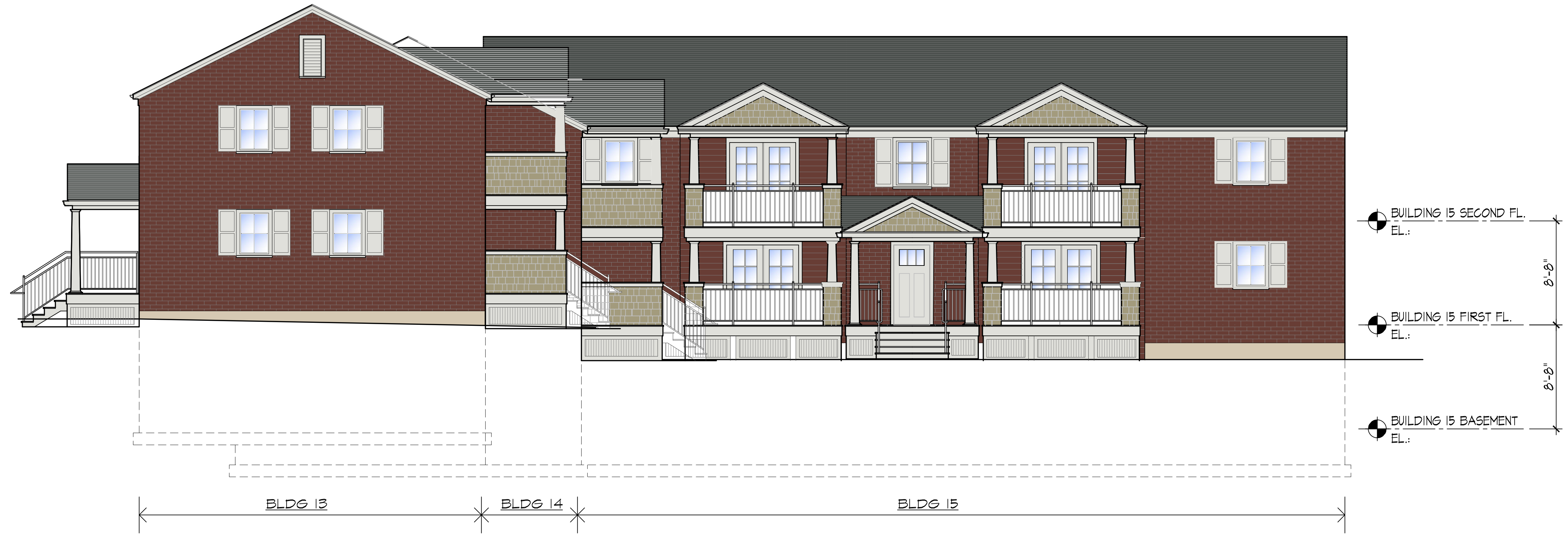
2 SOUTH ELEVATION BUILDING # 6 A2.1B6 1/8"=1'-0"
