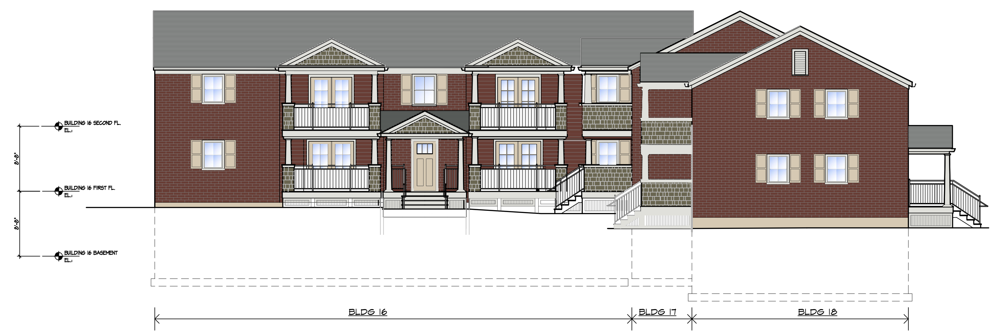
2 NORTH ELEVATION BUILDING # 4 A2.2B4 1/8"=1'-0"
