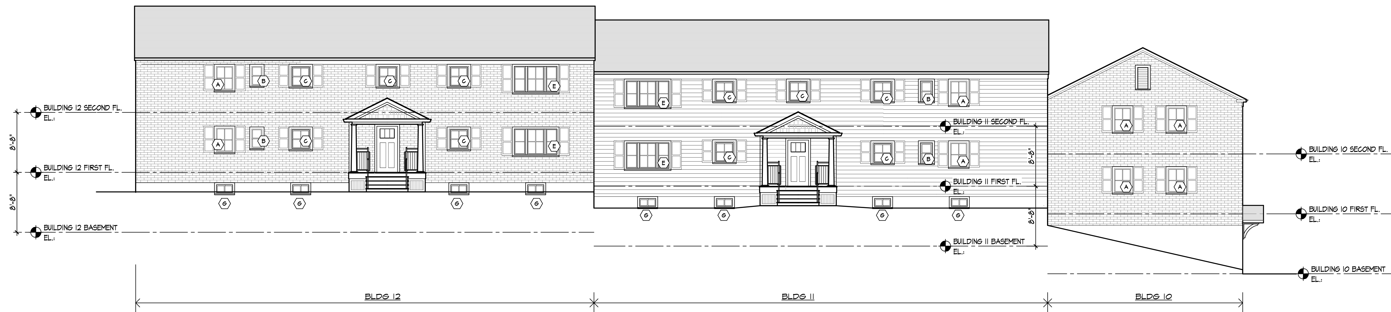
2 SOUTH ELEVATION BUILDING #7 A2.1B7 1/8"=1'-0"
