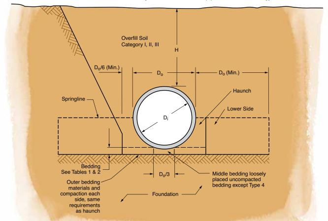
There are four types of Standard Installations, each with its own soil and compaction requirements. Type 1 bedding provides the most support using highly compacted granular material, while Type 4 provides for less support allowing the use of silts and clay soils with little or no compaction. These four choices provide flexibility and versatility for the designer and contractor, as well as performance and economy for the owner that are not available with other types of pipe.
