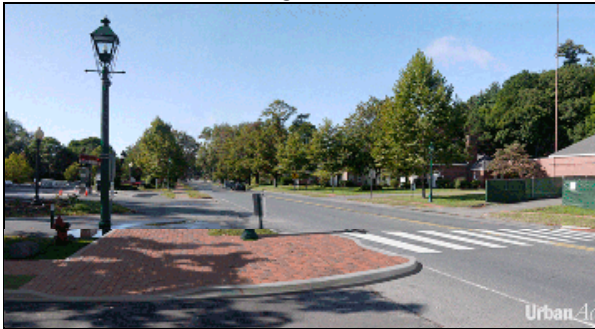
Addition of partial brick sidewalks, "bumpouts" to narrow travel lanes, and crosswalks
